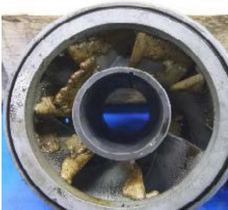
First stage of ESP with accumulation of scale at the impeller.
